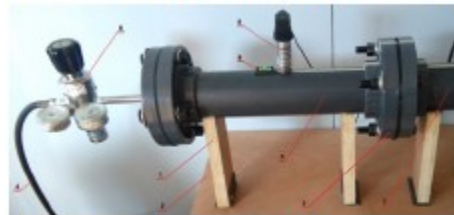
Figure 2. Shock tube prototype. High pressure camera (driver section).
