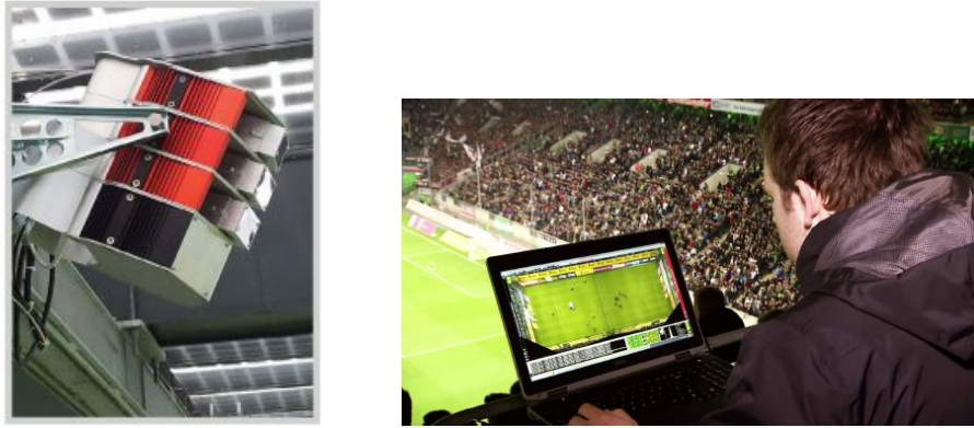
Figure 1.2: TRACAB Soccer Players Tracking System: Camera array and supervised real time tracking. Source: https://chyronhego.com/products/sports-tracking/tracab-optical-tracking/
