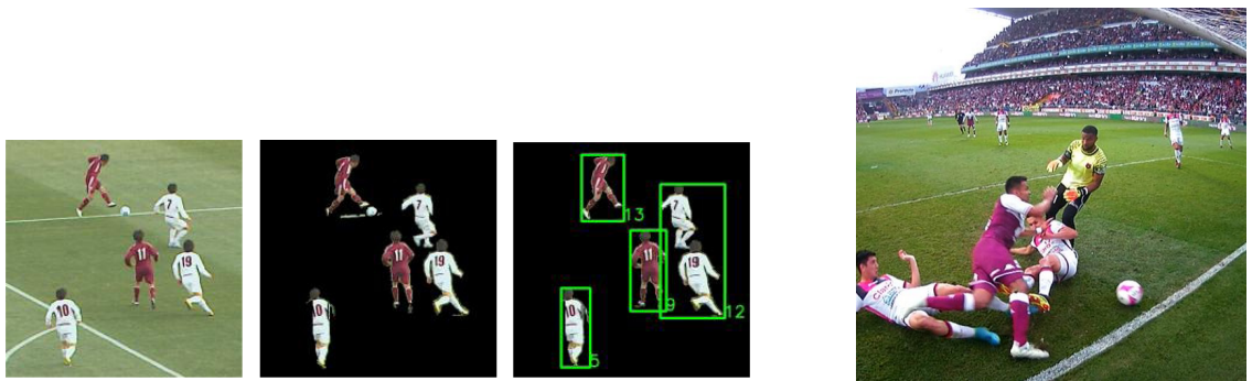
(a) Minimum proximity between players is considered as an occlusion event by the algorithm, which groups both players as a single one. [74]
