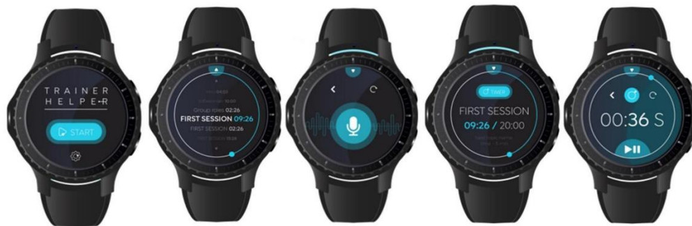
Fig. 6 Trainer Companion Screens. Left to right: Main screen, overall view of the agenda, recording functionality, session timer, and activity stopwatch
