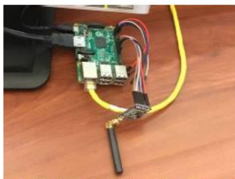
Fig. 14. Raspberry Pi 3 and RFM69HCW module used to collect scientific data.
