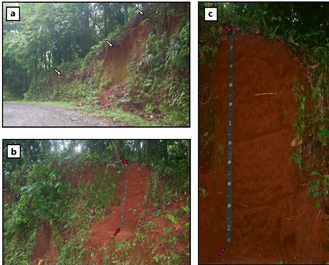
Fig. 21.19 Highly weathered soils in the Mountains of Tortuguero-Barra del Colorado: a Road cut that extends along the road to Barra del Colorado, exhibiting weathered reddish deep soils (white arrows);
