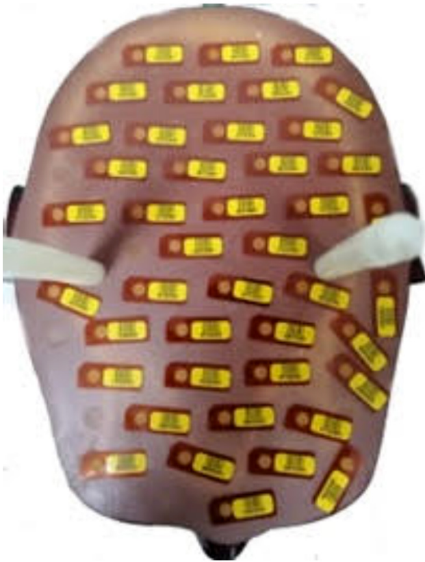
Figure 3. TLD dosimeters placed on one of the slices of the phantom.
