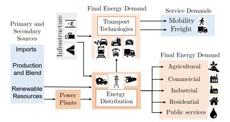
Figure 2.2: Reference Energy System (RES) of OSEMOSYS-CR.
