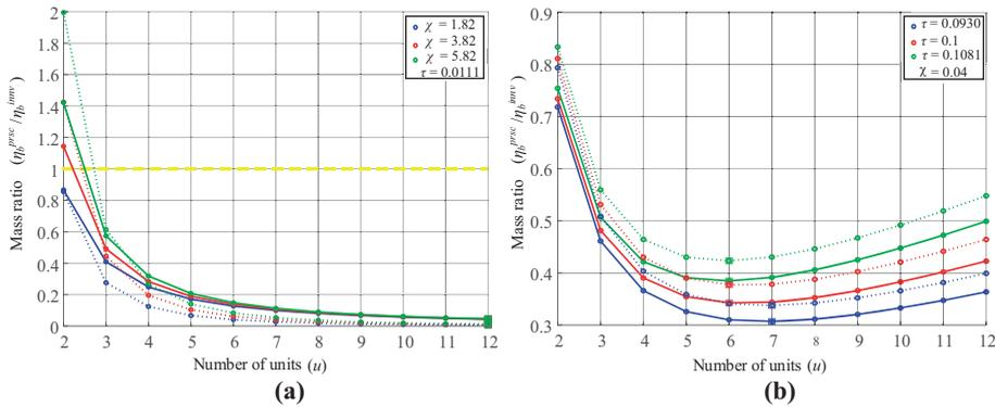
**Notes:** (a) Simulated mass ratio considering the variable  $\tau$  fixed; (b) mass ratio of prismatic and innovative tensegrity with variable  $\chi$  fixed. The dotted lines represent the regressive curve of  $\eta_b^{inv}$ , and the continuous lines represent  $\eta_b^{prsc}$
