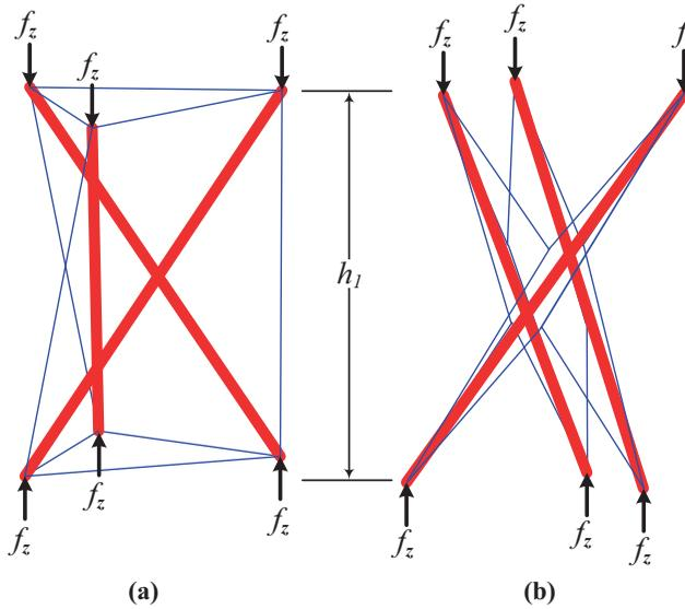
**Notes:** (a) Three struts prismatic tensegrity under a compressive force  $f$ ; (b) a compressed three struts innovative tensegrity by a force  $f$ . The height of the structure is noted as  $h_1$  instead of  $h$
