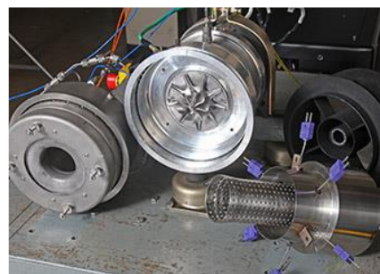
SwRI used a specialized 3D printer that can craft layered and highly detailed metal parts to build its radial gas turbine. Image: Southwest Research Institute
