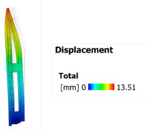
Fig. 5. Results of total displacement for each wing according to the simulation
