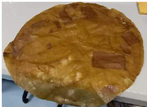
Fig. 13. Patched biotextile parachute for real size model
