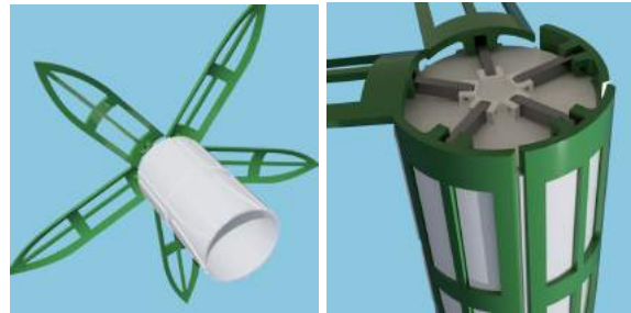
Fig. 4. Detail of the opening mechanism for the prototype
