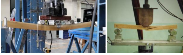
Figure 6: Bending test structural size (left) and defect free specimen (right).
