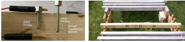
Figure 4: Monitoring of internal MC and internal temperature with sensors inserted inside the wood.
