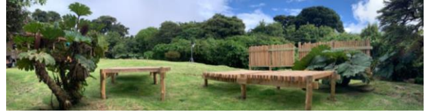
Figure 2: Experimental specimens exposed above-ground to environments with different degrees of acidic atmospheres
