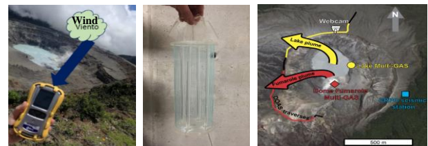
Figure 3: Multirae gas monitoring, acid rain from fog collector image on the right adapted from [35].
