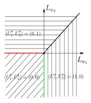
Figure 5: Phase plane of switching functions.
