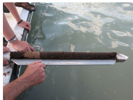
A sediment core taken from a coastal lagoon in Sian Kaan, Mexico, containing a clastic layer probably deposited by a hurricane (Photo credit: J. Donnelly)
